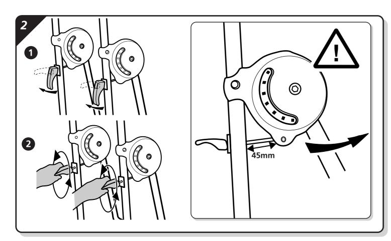
(1) Release the two carrier clamping levers and (2) turn the handles anti-clockwise until the angle adjusters are fully opened,
